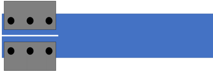
Figure 2.9: DCB test specimen geometry.
