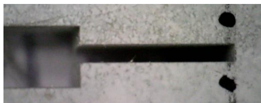
Figure 3.16: Square shaped notch tip of CT specimen.
