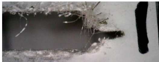
Figure 3.24: Round shaped notch tip of WCT specimen.
