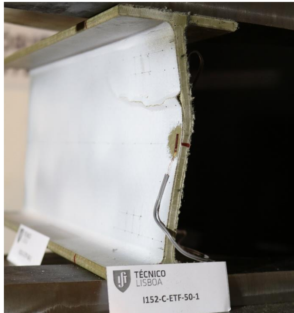
Figure 6.7: Web-buckling failure mode of I152-C-ETF-50-1 specimen.
