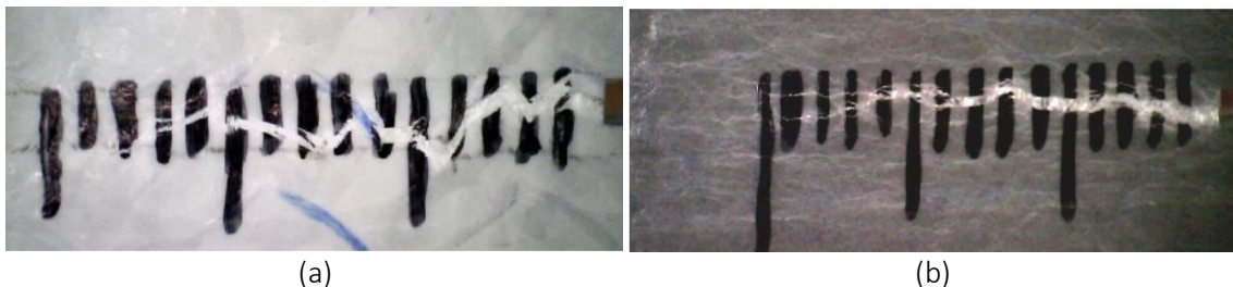
Figure 4.5: Crack growth patterns in CT test specimens (scale marker used to validate measurements from microscopic camera): (a) P300-A-CT-23-3; (b) I150-S-CT-18-3.
