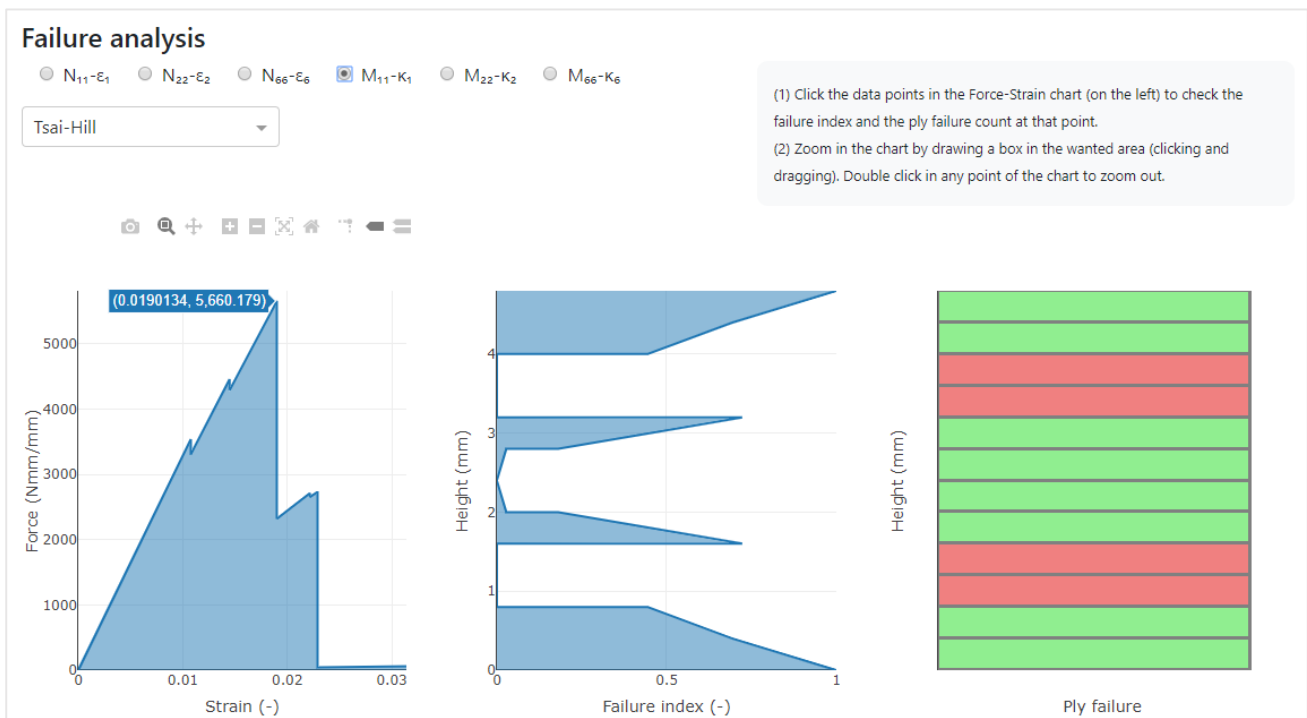
Figure 24 – Force-strain progressive failure path chart, failure index chart and lamina discount chart (in this illustrative example M_{11}-\kappa_1 ).
