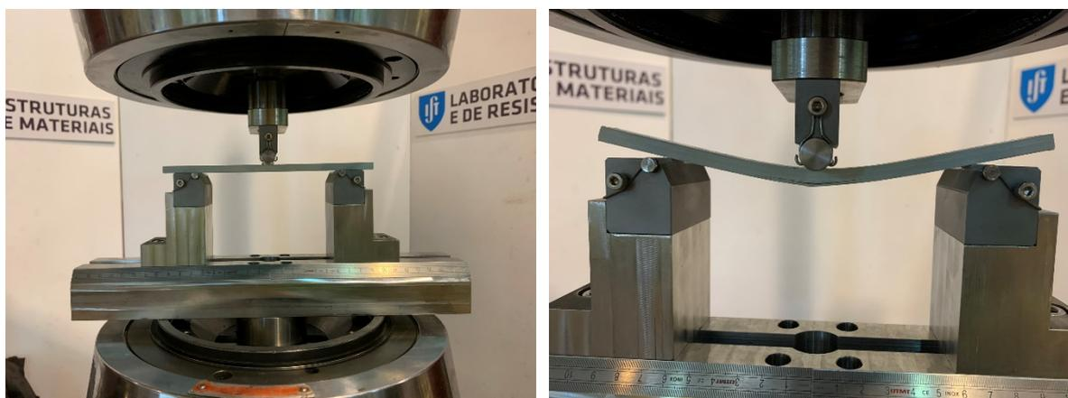
(a) Flexural test setup
