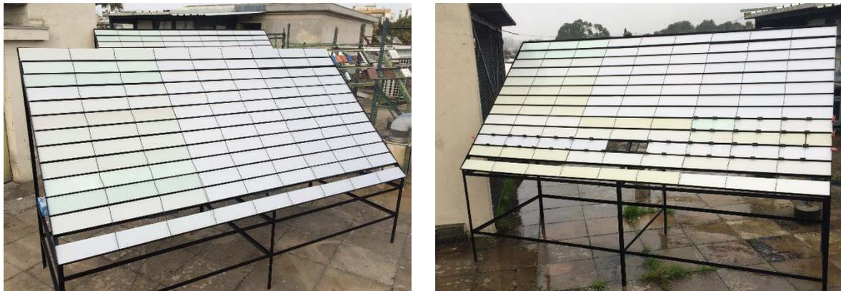
**Figure 13.01 - Structure for natural weathering exposure (LNEC rooftop).**
