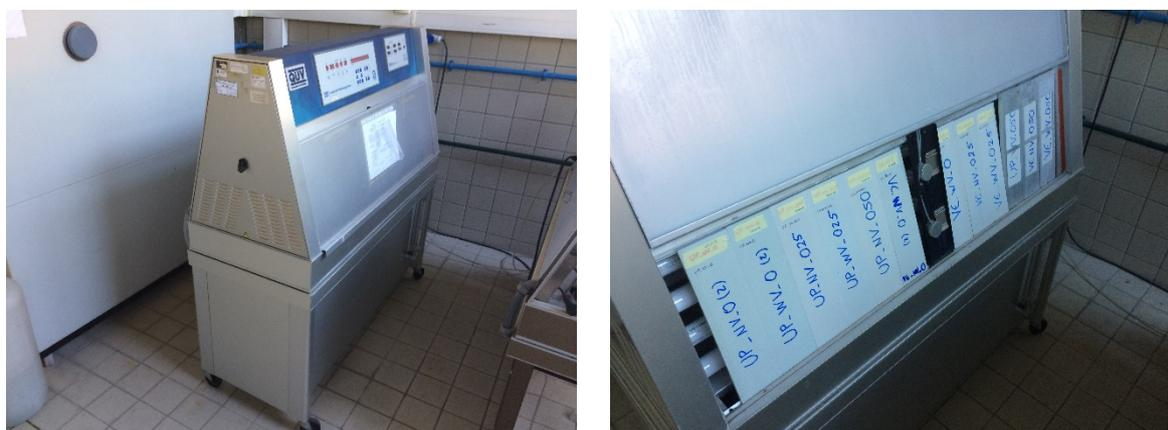
**Figure 13.03 - QUV chamber (LNEC laboratory).**
