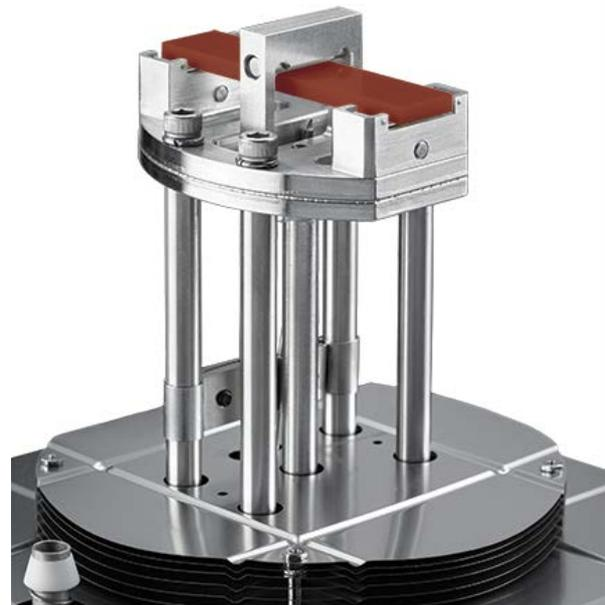
Three-point bending test setup
