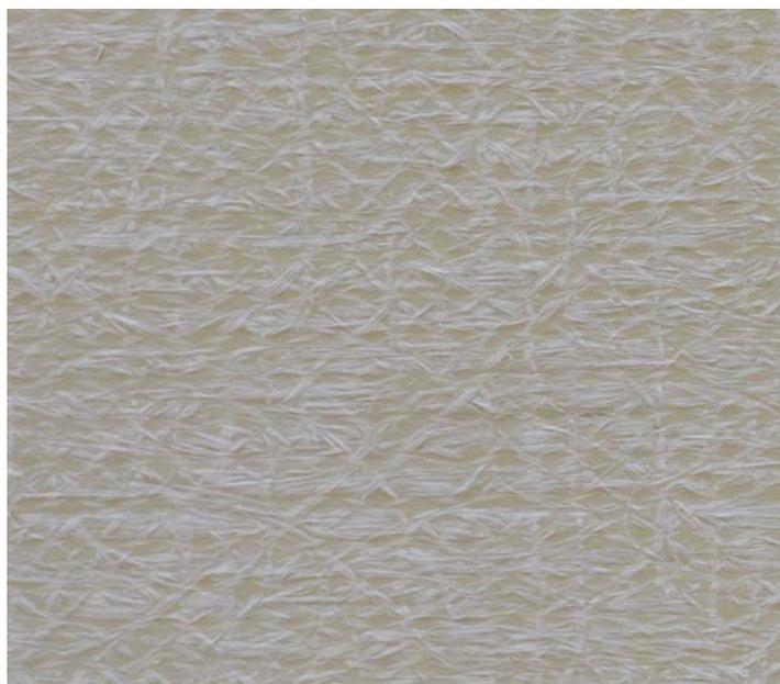
(b) Picture of the above specimen after the software analysis (49.5% image area of fibres)
