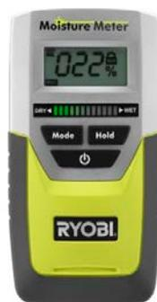
**Figure 6.04 - Moisture meter (adapted from [II.33]).**
