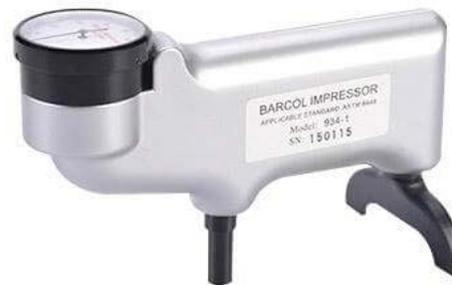
**Figure 6.01 - Barcol impressor (adapted from [II.31]).**
