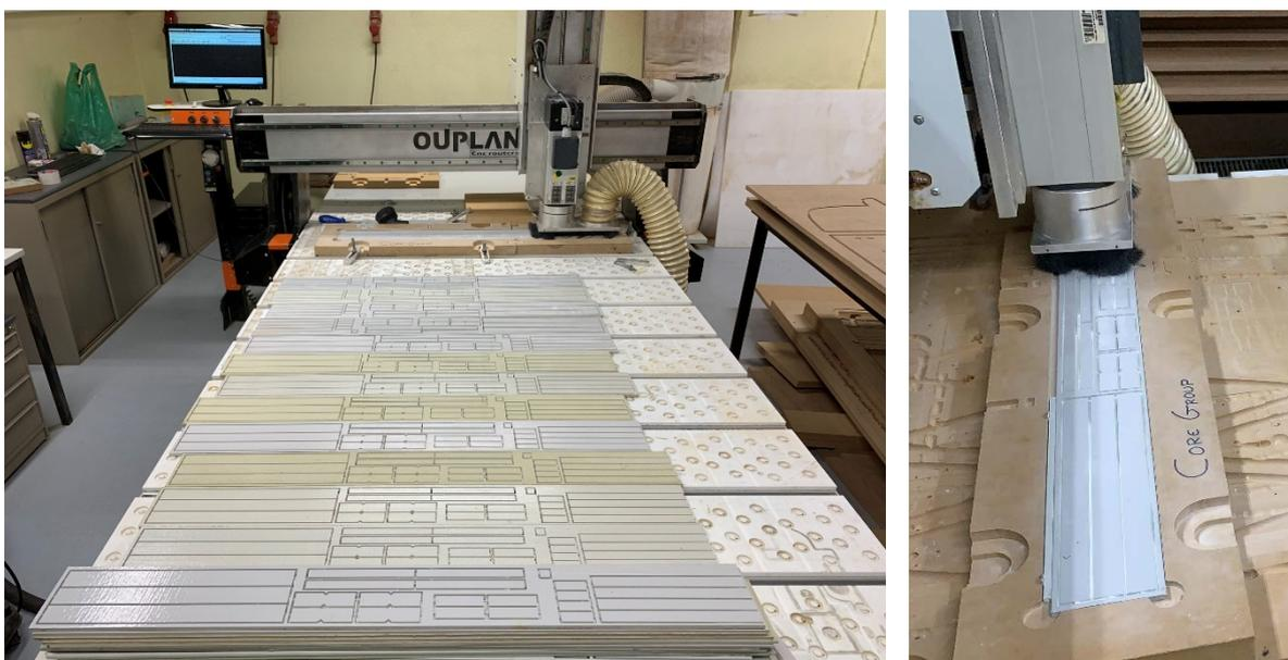
**Figure 11.02 - CNC cutting machine used for specimen cutting.**
