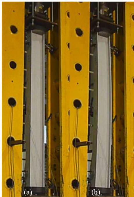
*Figure 4.18: Typical limit state of long columns: (a) undeformed shape, and (b) deformed shape.*
