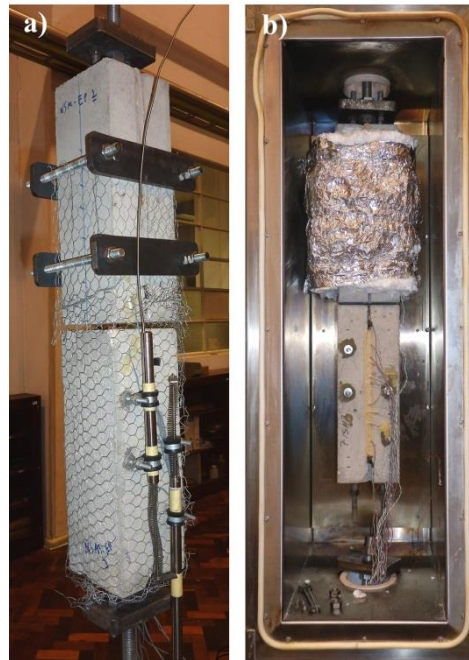
Figure 3.20: Setup for tests at a) ambient temperature and b) elevated temperature.
