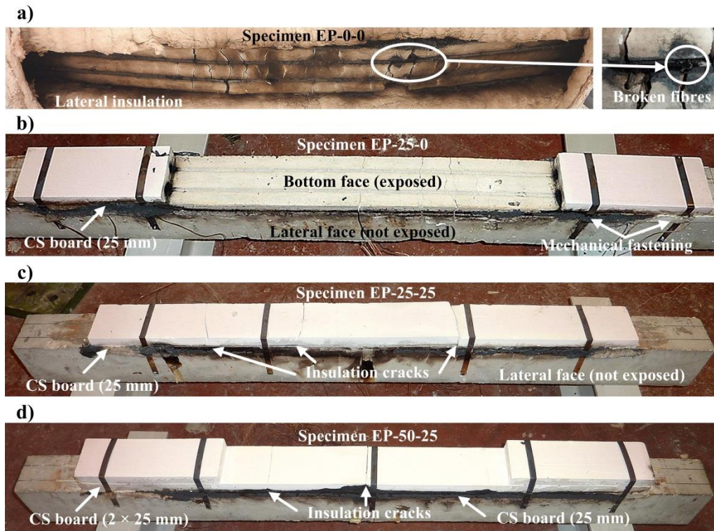
Figure 7.14: Post-fire observations: a) beam EP-0-0; b) beam EP-25-0; c) beam EP-25-25; d) beam EP-50-25.
