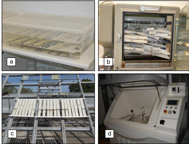
Figure 10.5. Ageing environments: (a) immersions, (b) continuous condensation, (c) natural ageing, (d) salt fog spray.
