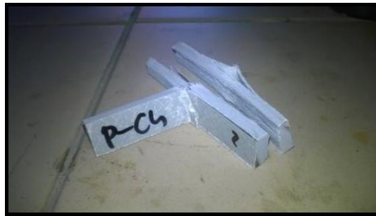
Figure 12.9. Partial failure modes observed in the Charpy shock test.
