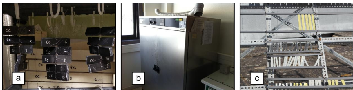
Figure 9.3. Ageing environments: (a) condensation chamber, (b) chamber used for immersions; (c) natural exposure in LNEC's roof.
