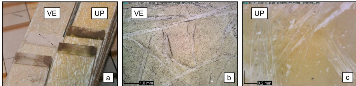
Figure 5.8. (a) Fibre blooming effect after 102 months of natural exposure; (b) VE profile 50 \times magnification; (c) UP profile 220 \times magnification.
