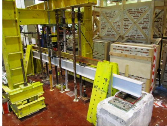
Figure 4.47.: Full-scale flexural failure tests: test setup of the I200 specimen.
