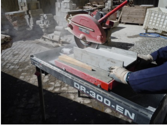
Figure 4.1.: Extracting coupons: separating the flanges from the web.
