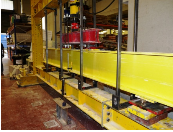
Figure 4.71.: Full-scale flexural tests: failure mode of specimen P400-3, global view.
