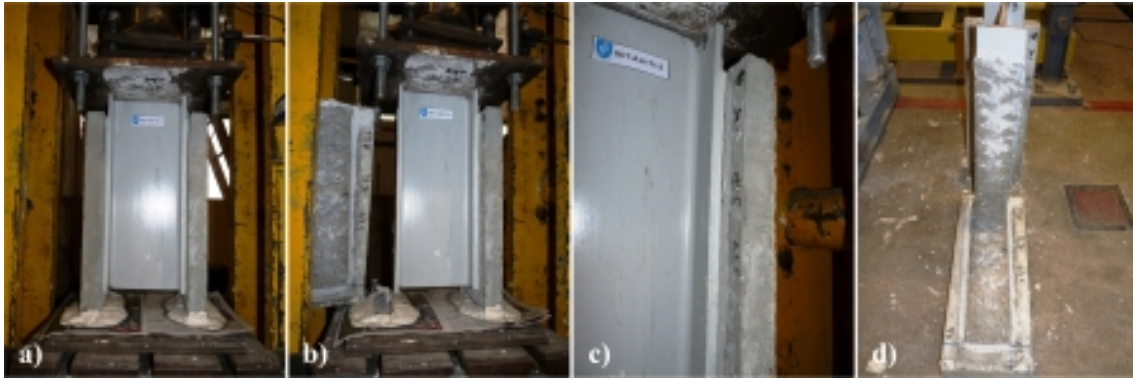
Figure 5.61.: Specimen A-H-T1-3: a) beginning of the test; b) collapsed specimen; c) incomplete debonding; d) failure surfaces.
