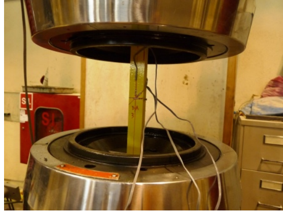
Figure 4.26.: Coupon off-axis tensile tests: I400 specimen.
