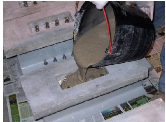
Figure 5.20.: Preparation of the bolted specimens: filling of the negatives with epoxy mortar.
