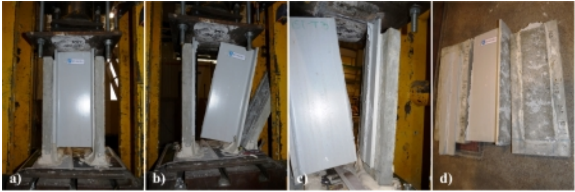
Figure 5.67.: Specimen A-H-T3-1: a) beginning of the test; b) collapsed specimen; c) web-flange junction failure; d) failure surfaces.
