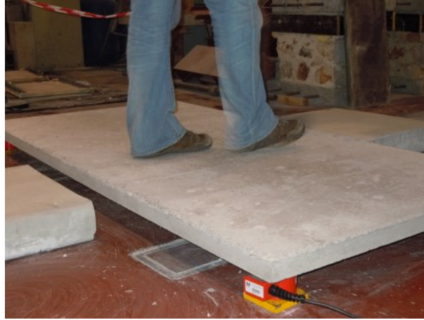
Figure 6.64.: Pedestrian induced actions: experimental evaluation of load-time functions.
