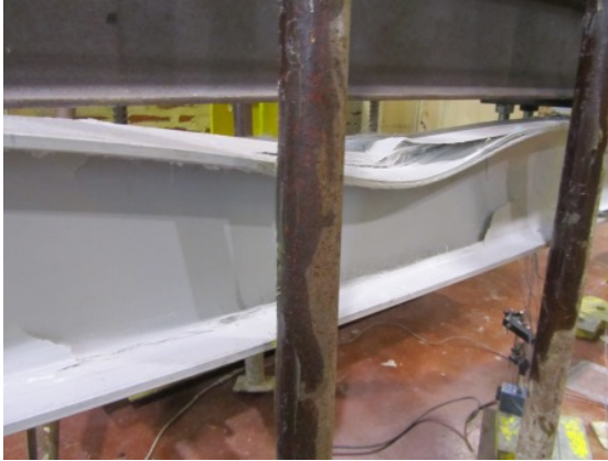
Figure 4.50.: Full-scale flexural failure tests: configuration of the local buckling wave in the I200 profile (near one of the loading sections).
