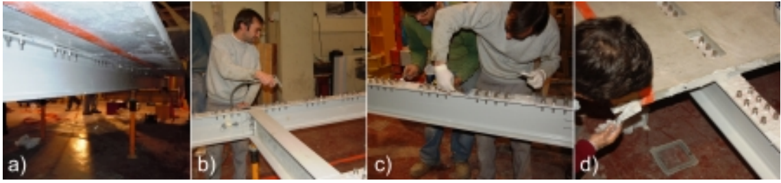
Figure 6.29.: Bonding of the elements: a) preamber props; b) dusting of the surface; application of the adhesive on the c) main girders; and d) on the SFRSCC slabs.
