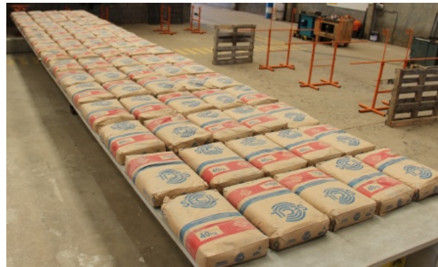
Figure 7.53.: Full-scale prototype loaded in the creep test.
