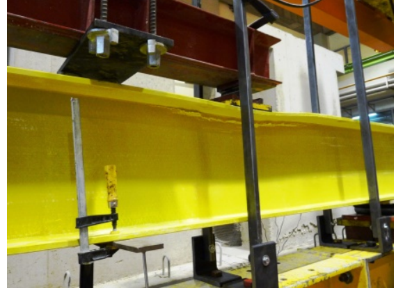
Figure 4.72.: Full-scale flexural tests: failure mode of specimen P400-3, damage on the web-flange junction.
