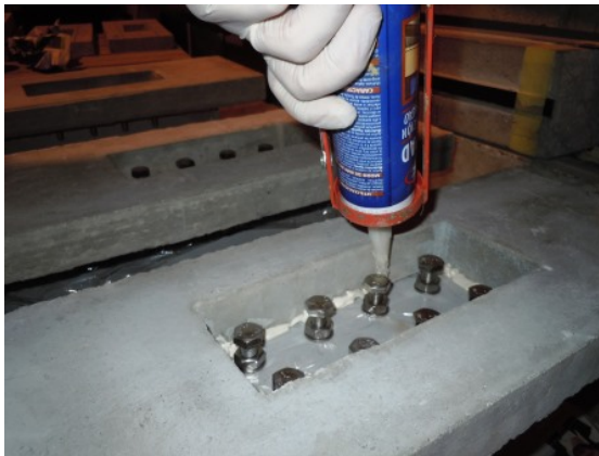
Figure 5.19.: Preparation of the bolted specimens: sealing of the GFRP-SFRSCC joints (M series only).
