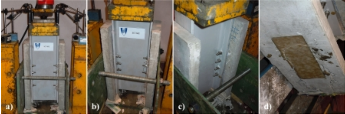
Figure 5.44.: Specimen M-2: a) beginning of the test; b) deformation of the bolts; c) crushing of the GFRP flanges; d) damage on the SFRSCC (after failure).
