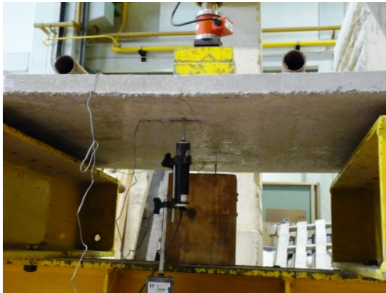
Figure 4.94.: Flexural tests on SFRSCC slabs: initial crack opening.
