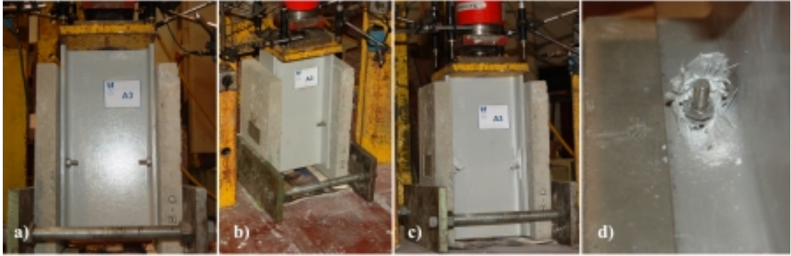
Figure 5.28.: Specimen P-M1-2: a) beginning of the test; b) beginning of the crushing, and of bolts' deformation; c) failure due to crushing of the flange; and d) detail of the interaction between the bolts and the profile.
