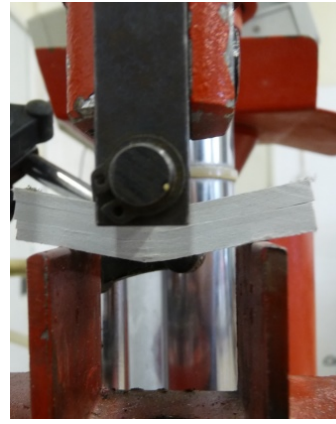
Figure 4.37.: Coupon interlaminar shear test after specimen failure.
