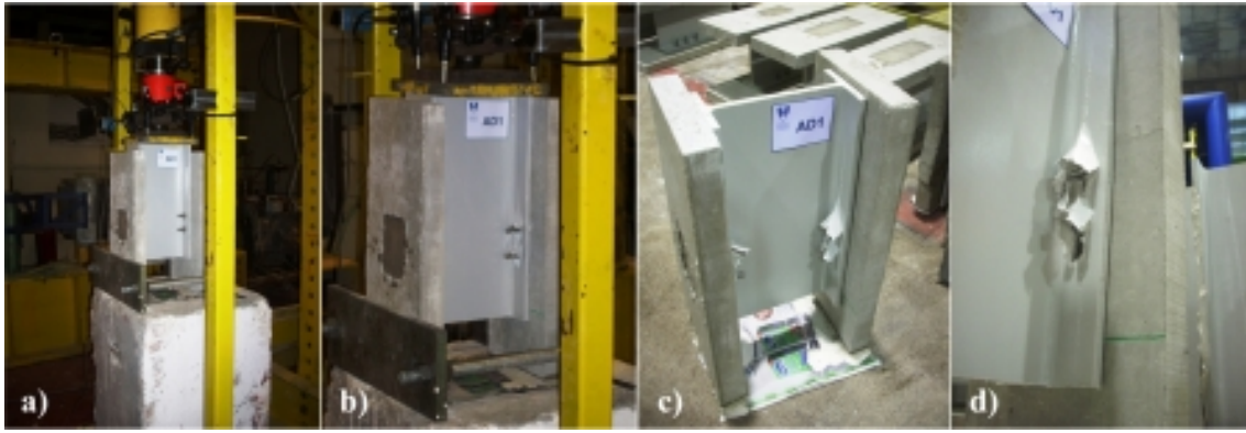
Figure 5.30.: Specimen P-M2-1: a) beginning of the test; b) deformation on the bolts/beginning of GFRP flange crushing on the GFRP flange; c) collapsed specimen; d) detail of the GFRP flange crushing.
