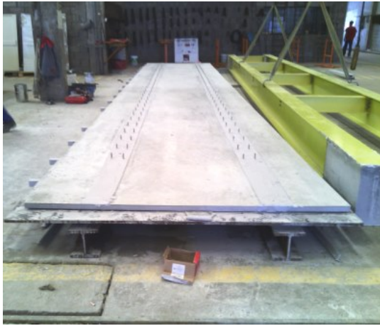
Figure 7.19.: Application of the epoxy adhesive layer.
