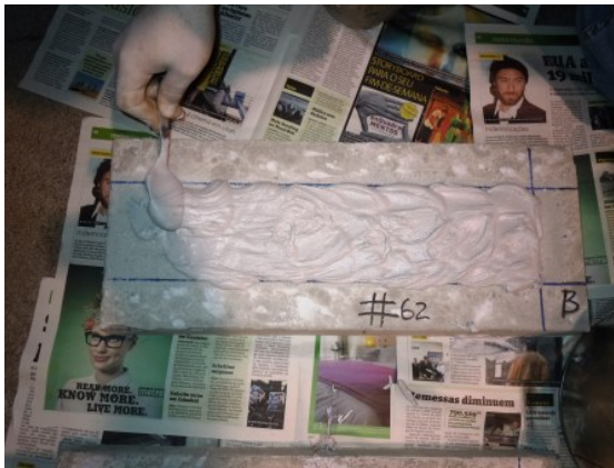
Figure 5.11.: Preparation of the adhesively bonded specimens: application of the resin.
