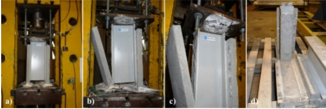
Figure 5.50.: Specimen A-Th-T1-2: a) beginning of the test; b) collapsed specimen; c) debonding failure in the SFRSCC; d) debonded surfaces.
