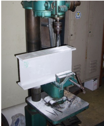
Figure 5.15.: Preparation of the bolted specimens: drilling of the profiles.
