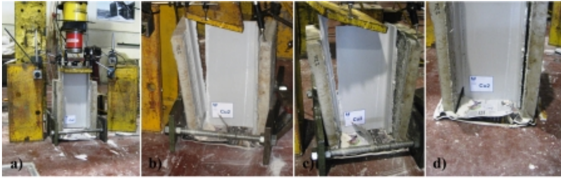
Figure 5.26.: Specimen P-A-6: a) beginning of the test; b) failure of the specimen; c) detail of the web-flange junction failure — complete separation; and d) detail of the failure at the interface — complete separation.
