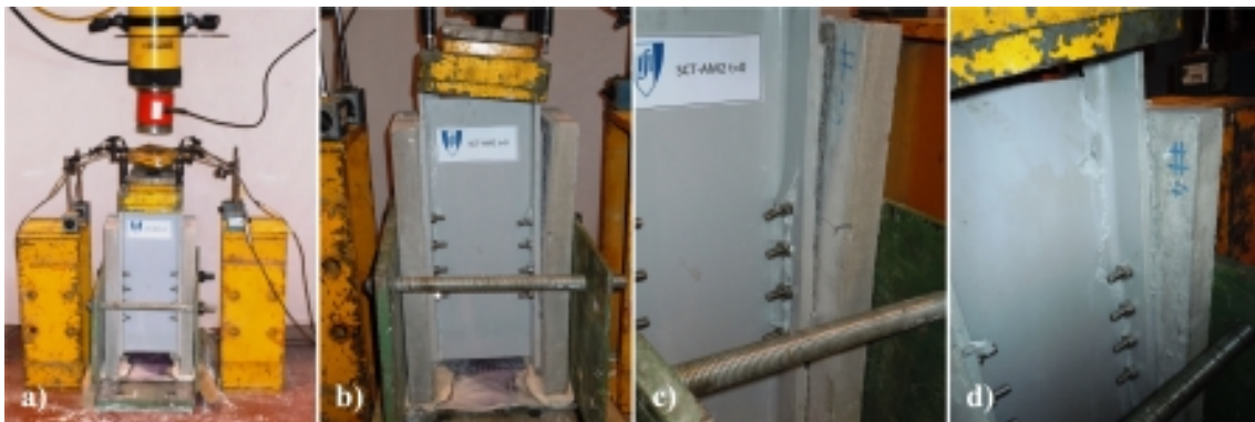
Figure 5.46.: Specimen AM-2: a) beginning of the test; b) collapsed specimen; c) debonding and crushing of the flange; d) web-flange junction failure.
