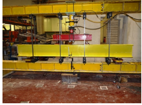
Figure 4.59.: Full-scale flexural failure tests: I400 profiles — test setup for the shorter specimen.
