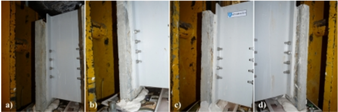
Figure 5.68.: External signs of fibre corrosion in AM-H-T3 series, specimens: a) AM-H-T3-1; b) AM-H-T3-2; c) AM-H-T3-3; d) AM-H-T3-3.
