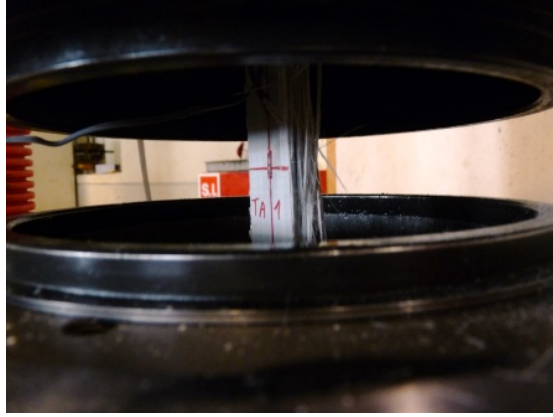
Figure 4.9.: Coupon tensile tests: failure mode of I200 specimens.
