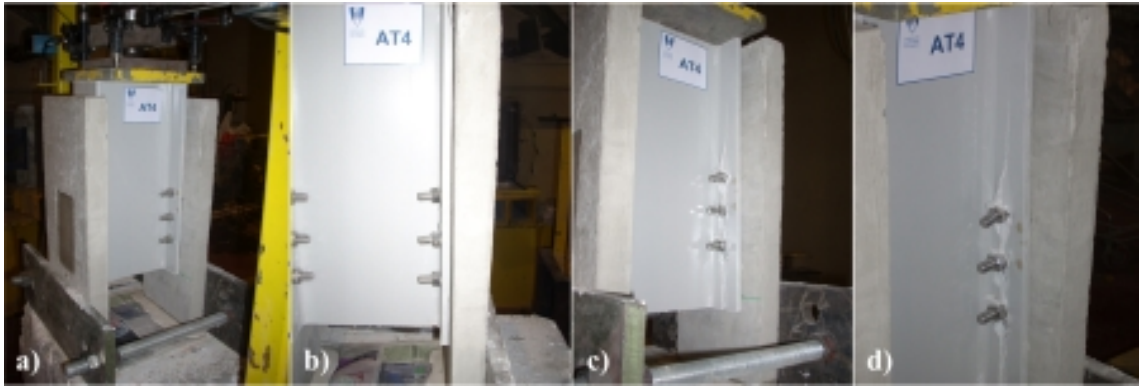
Figure 5.32.: Specimen P-M3-4: a) linear stage; b) non-linear stage (deformation of the bolts on the left side only); c) crushing of the GFRP flange; d) crushing of the GFRP flange — detail.
