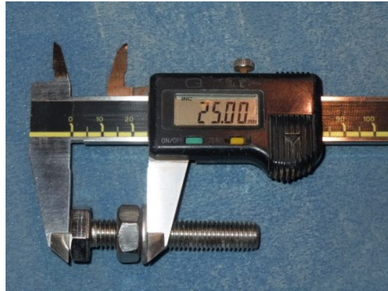
Figure 5.16.: Preparation of the bolted specimens: embedded length of the connectors.
