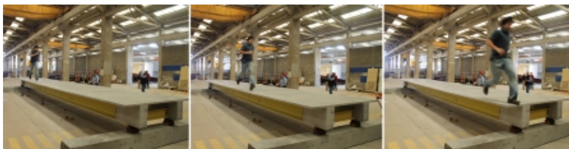
Figure 7.37.: Full-scale prototype one pedestrian tests: pedestrian running in the eccentric path.
