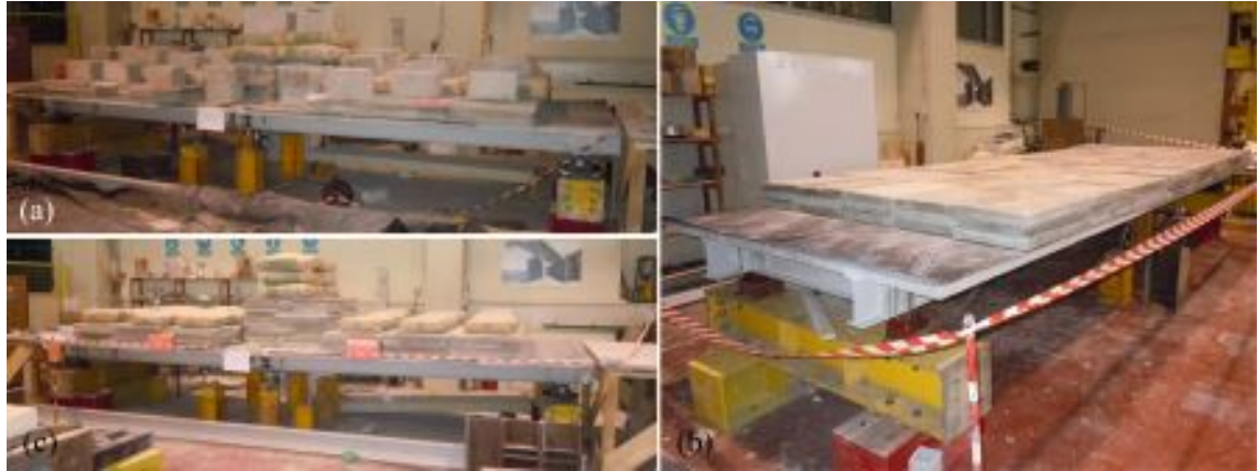
Figure 6.86.: Small-scale prototype loaded for creep test: a) test 1; b) test 2; and c) test 3.
