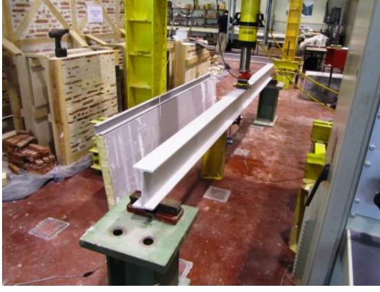
Figure 4.40.: Full-scale flexural serviceability tests: test setup for the I200 profile.
