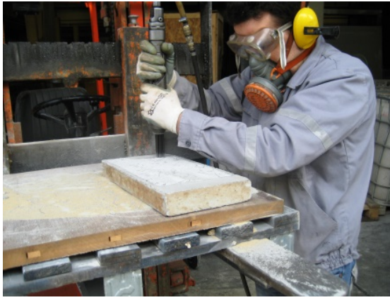
Figure 5.9.: Surface preparation of a SFRSCC slab for the adhesive bonding.
