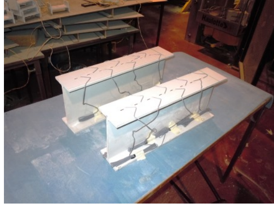
Figure 5.14.: Preparation of the adhesively bonded specimens: specimens instrumented with strain gauges.
