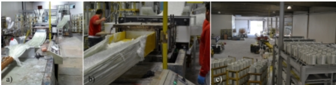
Figure 2.19.: Pultrusion of an I-shape profile: a) pulling of the dry fibres; b) first stretch of cured FRP; and c) general view of the pultrusion line.
