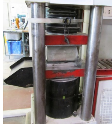
Figure 4.89.: Splitting tensile strength tests on SFRSCC cylinder specimens.
