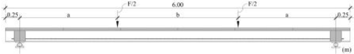
Figure 6.37.: Small-scale prototype serviceability tests: load configuration 2.
