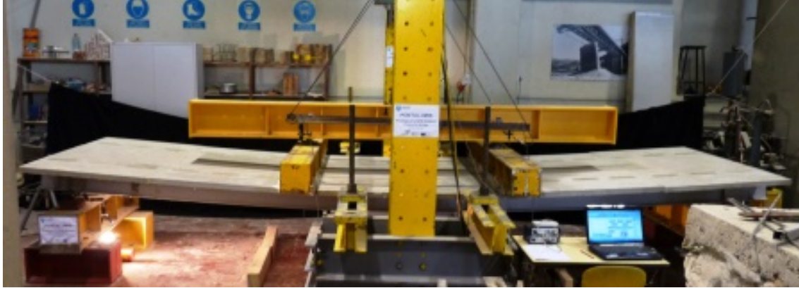
Figure 6.45.: Small-scale prototype failure test: deformed configuration immediately prior to failure.
