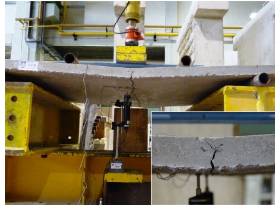
Figure 4.95.: Flexural tests on SFRSCC slabs: crack opening in the brink of failure (overall and detail views).
