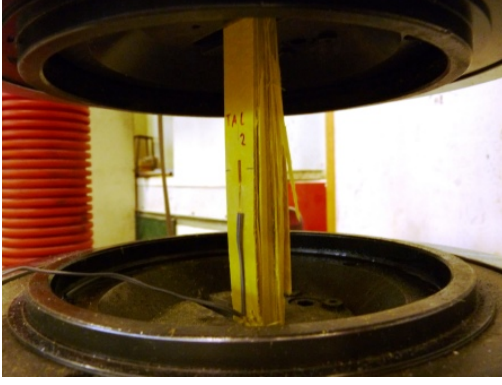
Figure 4.13.: Coupon tensile tests: failure mode of I400 specimens tested in the longitudinal direction.
