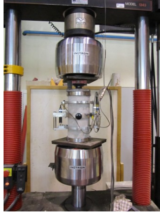
Figure 4.88.: Compressive tests on SFRSCC cylinder specimens.
