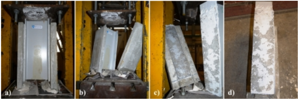
Figure 5.64.: Specimen A-H-T2-3: a) beginning of the test; b) collapsed specimen; c) failure surfaces; d) debonding in the epoxy resin.
