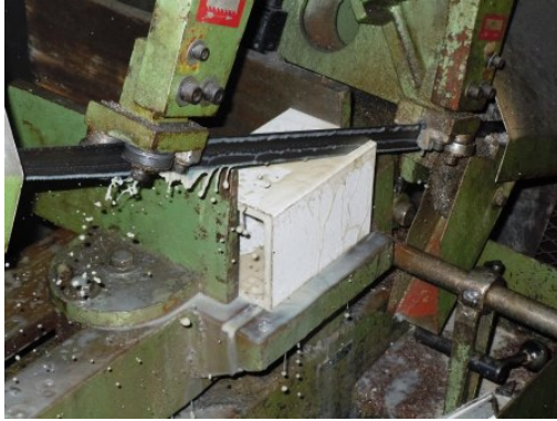
Figure 6.22.: Cutting of the square-section profiles.
