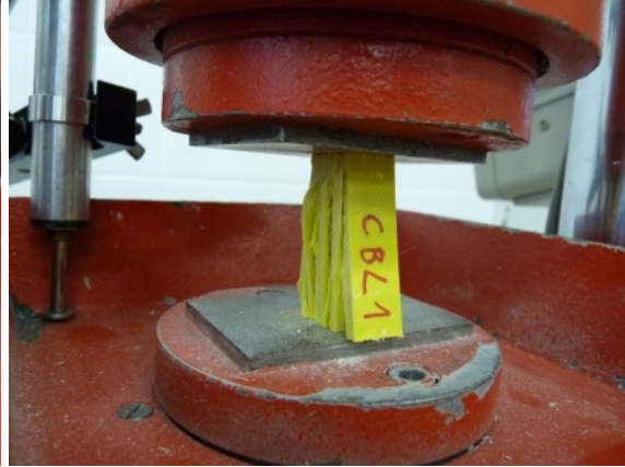
Figure 4.16.: Coupon compressive tests: I400 specimen.
