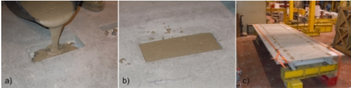
Figure 6.33.: Sealing the negatives: a) pouring the epoxy mortar; b) sealed negative; and c) final aspect of the prototype.
