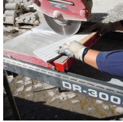
Figure 4.2.: Extracting coupons: cutting off-axis coupons.
