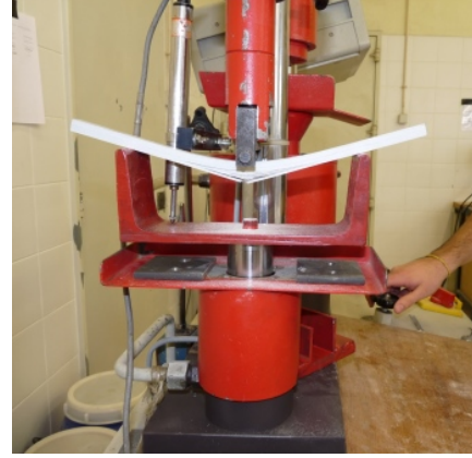
Figure 4.33.: Coupon flexure test after specimen failure.
