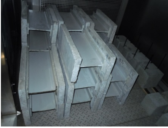
Figure 5.7.: Thermal cycle aging: specimens inside the climate chamber.
