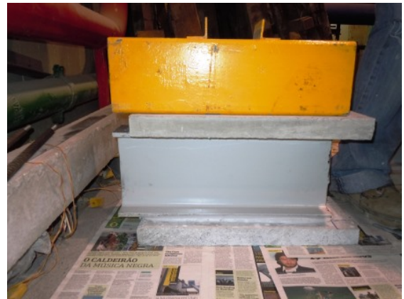
Figure 5.12.: Preparation of the adhesively bonded specimens: application of the weight.
