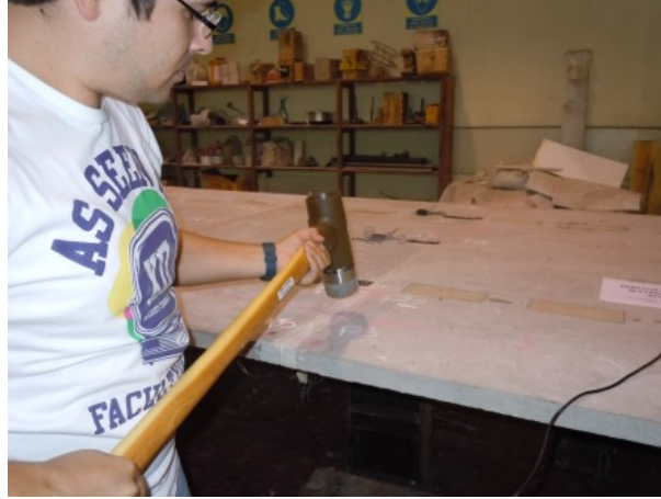
Figure 6.57.: Small-scale prototype modal identification tests: example of impact load being applied.
