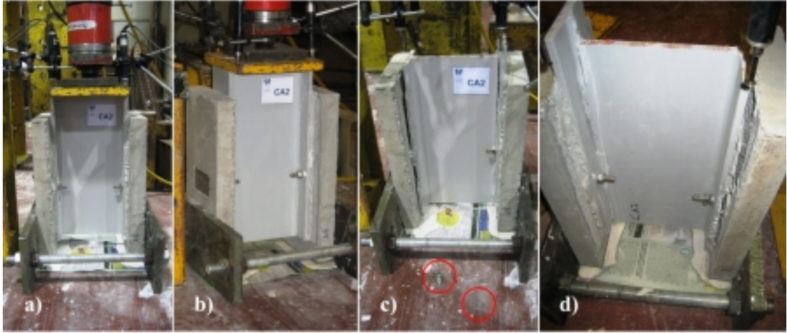
Figure 5.36.: Specimen P-AM-2: a) beginning of the test; b) failure of the web-flange junction; c) failure of the SFRSCC-adhesive interface; d) failure of both bolts of the same flange.
