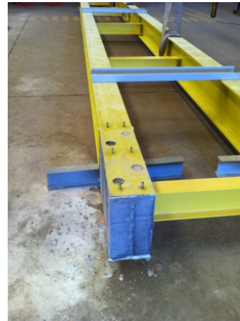
Figure 7.16.: Concrete jackets and stainless steel connectors.
