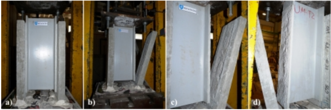
Figure 5.52.: Specimen A-Th-T2-3: a) beginning of the test; b) collapsed specimen; c) SFRSCC failure surface; d) GFRP failure surface.
