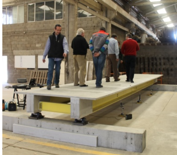
Figure 7.39.: Full-scale prototype crowd tests in progress.
