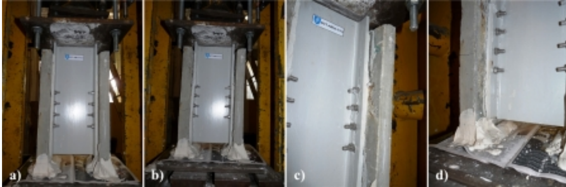
Figure 5.70.: Specimen AM-H-T3-3: a) beginning of the test; b) collapsed specimen; c) crushing of the flange; d) web-flange junction failure.
