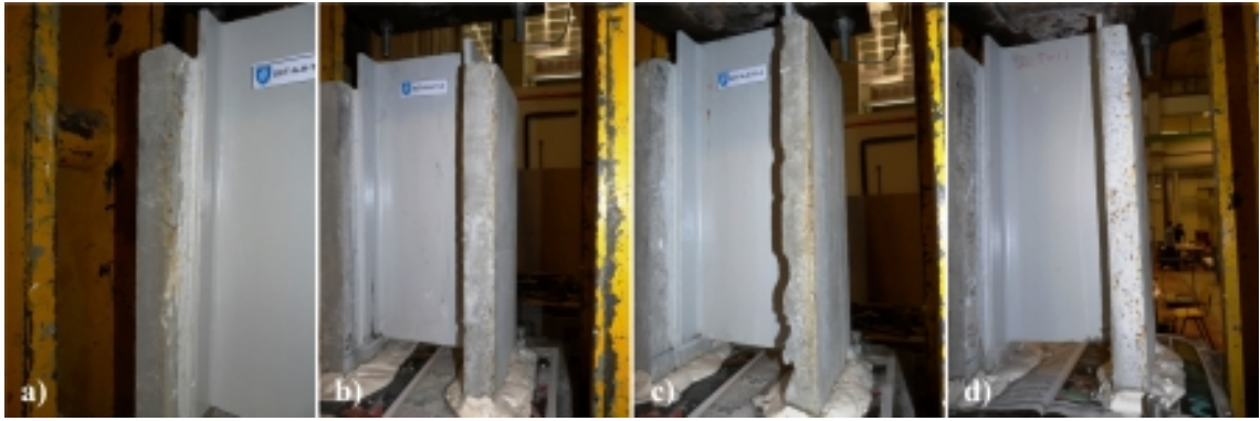
Figure 5.59.: External signs of fibre corrosion in A-H-T1 series, specimens: a) A-H-T1-2; b) A-H-T1-3; c) A-H-T1-4; d) A-H-T1-4.
