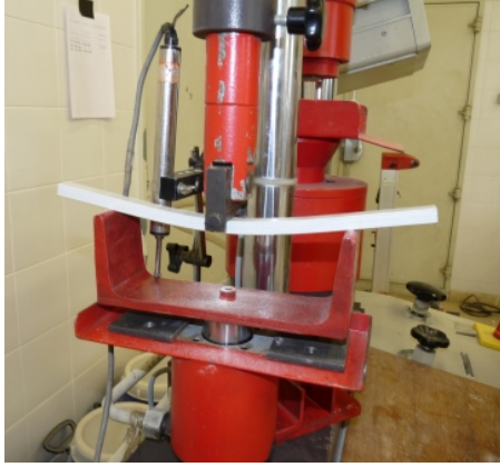
Figure 4.32.: Coupon flexure test before specimen failure.
