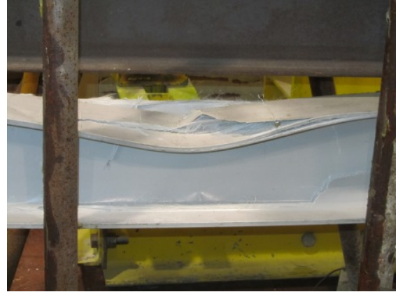
Figure 4.51.: Full-scale flexural failure tests: damage detail on the top flange and web of the I200 profile (near one of the loading sections).
