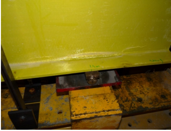
Figure 4.67.: Full-scale flexural tests: failure mode of specimen P400-1, front side view.
