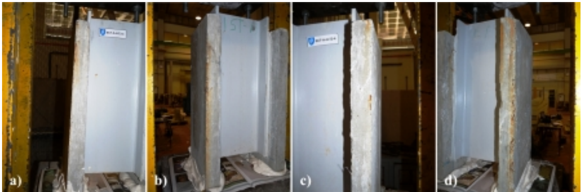
Figure 5.65.: External signs of fibre corrosion in A-H-T3 series, specimens: a) A-H-T3-3; b) A-H-T3-3; c) A-H-T3-4; d) A-H-T3-4.
