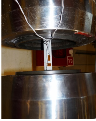
Figure 4.3.: Coupon tensile tests: I200 specimen.
