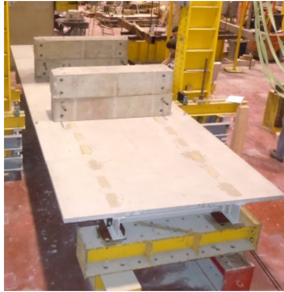
Figure 6.38.: Small-scale prototype serviceability tests: structure loaded in load configuration 2.
