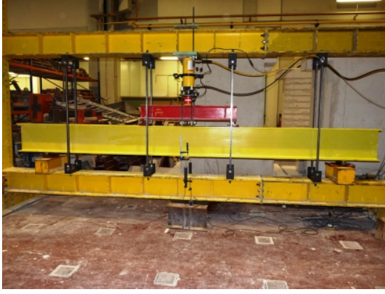
Figure 4.58.: Full-scale flexural failure tests: I400 profiles — test setup for the longer specimens.
