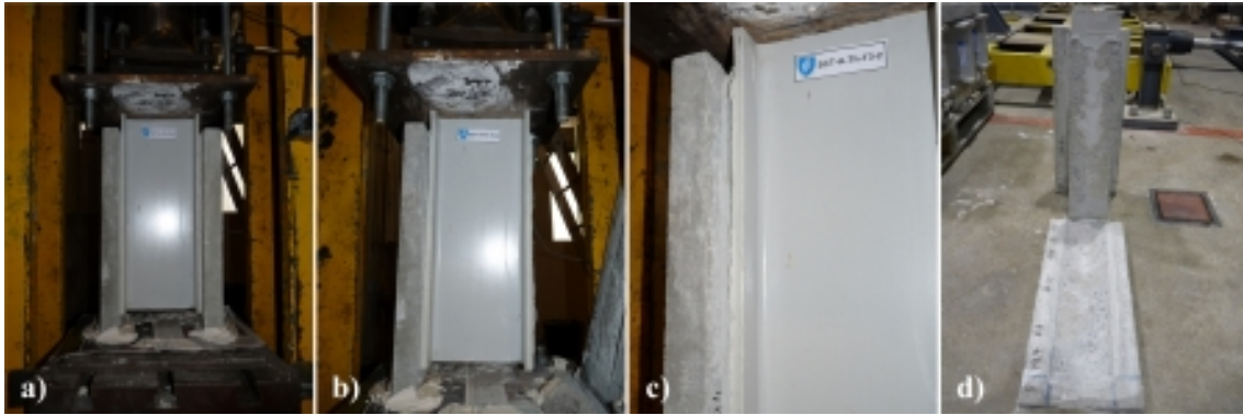
Figure 5.55.: Specimen A-Th-T3-2: a) beginning of the test; b) collapsed specimen; c) incomplete debonding; d) failure surfaces.
