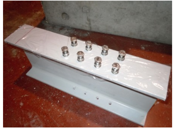
Figure 5.18.: Preparation of the bolted specimens: series M specimens provided with cellophane film.
