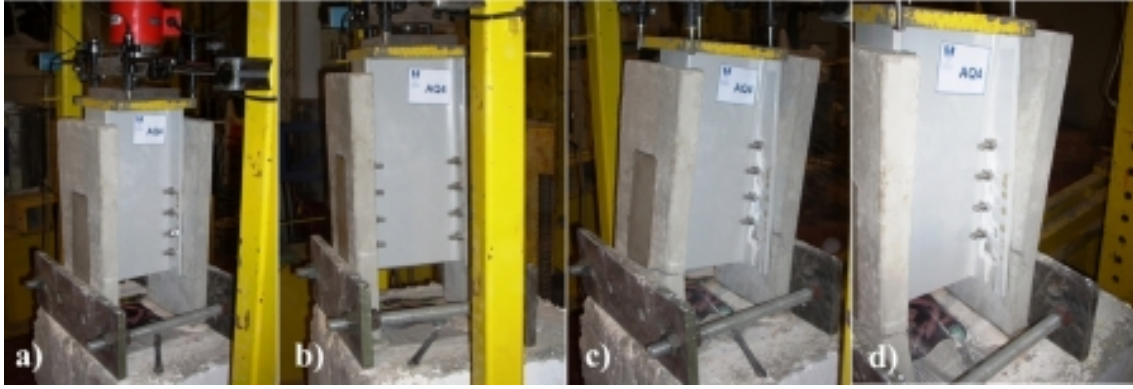
Figure 5.34.: Specimens P-M4-4: a) linear stage; b) non-linear stage — deformation of the bolts; c) collapsed specimen; and d) detail of the GFRP flange crushing.
