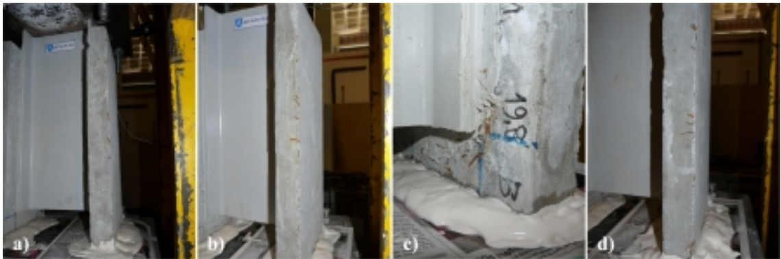
Figure 5.53.: External signs of fibre corrosion in A-Th-T3 series, specimens: a) A-Th-T3-1; b) A-Th-T3-2; c) A-Th-T3-4; d) A-Th-T3-7.
