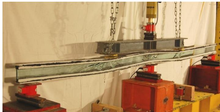
Fig. 6.20 - Crack pattern of beam *CS-I-SFlex-1* (before unloading).
