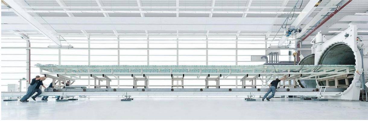
Fig. 2.2 – Processing of large-size glass elements at SEDAK [2.5].
