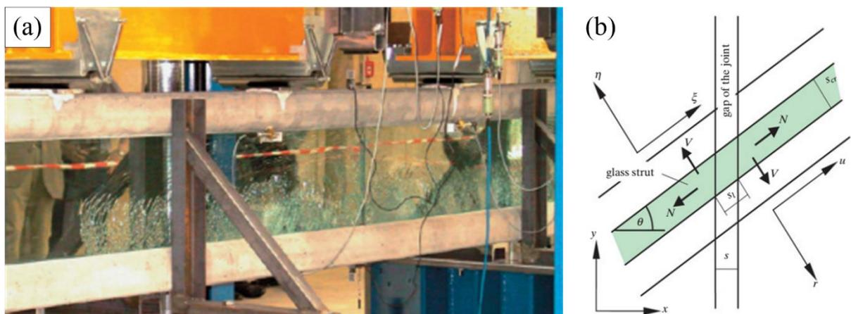
Fig. 2.24 – Glass-reinforced concrete hybrid beams: (a) flexural tests performed by Freytag and (b) analytical model considered [2.51].
