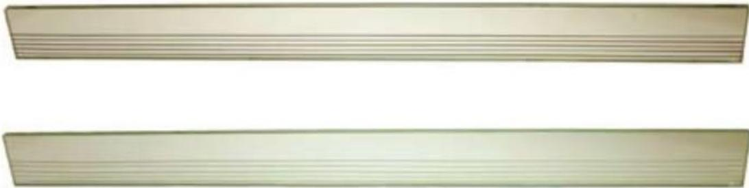
Fig. 2.27 - Reinforced glass beams with embedded (top) CFRP and (bottom) GFRP rods [2.55].
