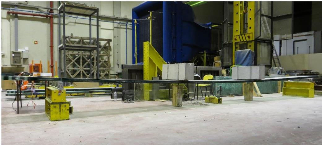
Fig. 4.3 – Flexural creep test of the SG panel.
