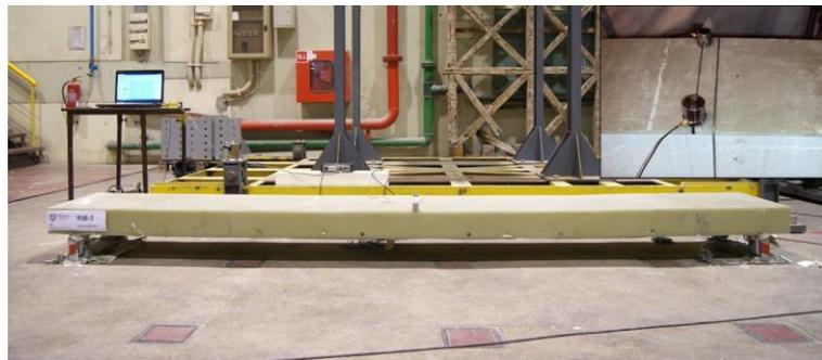
Figure 5.3. Experimental setup used for the dynamic tests.
