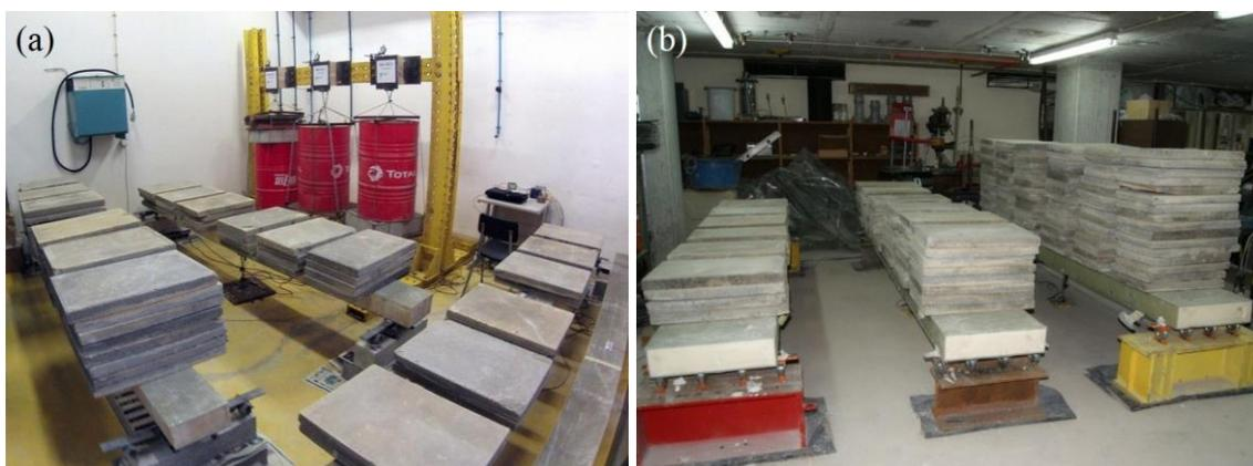
Figure 10.2. Full-scale creep tests setups for: (a) PUR, PET and BAL panels, and (b) RIB panels.
