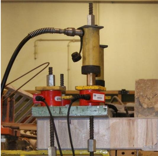
Figure 6.4. Support anchoring system for the cantilever tests.
