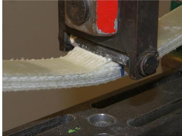
Figure 9.2. Typical flexural failure of the GFRP laminates.
