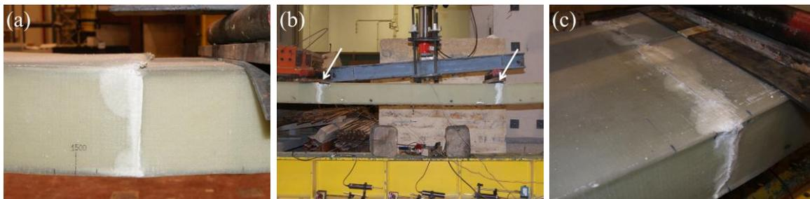
Figure 6.14. Failure of the ribbed panels in four-point bending: (a) failure at geometrical imperfection, (b) general view of failure at the loading points, and (c) detail of top face sheet and rib after failure at loading point.
