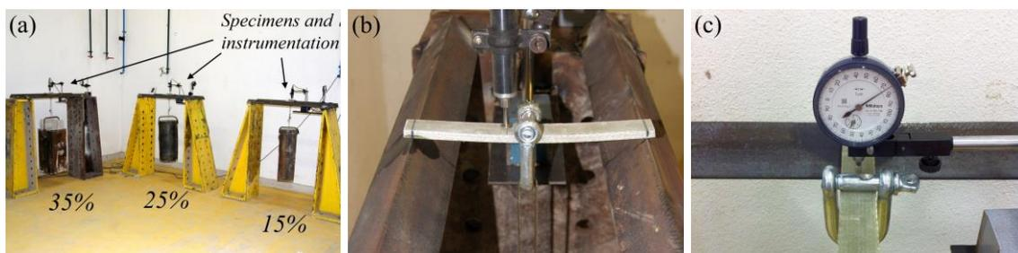
Figure 9.3. Flexural creep tests: (a) general view, (b) detail of specimen, and (c) dial gauge indicators.
