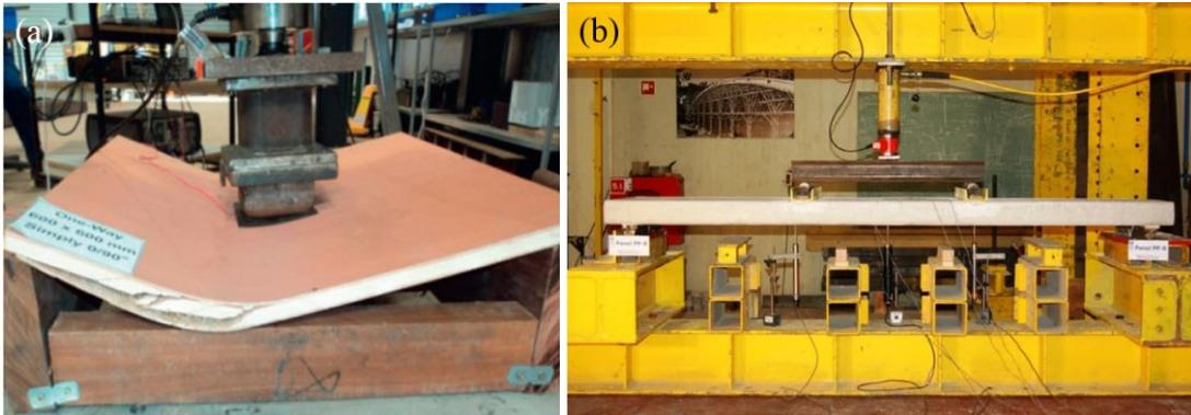
Figure 2.7. Sandwich floor panels: (a) deck panels [12], and (b) slab panels [13].
