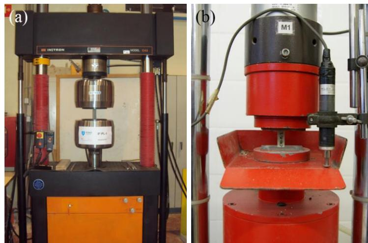
Figure 4.1. Experimental setups for the: (a) tensile tests, and (b) compression tests.
